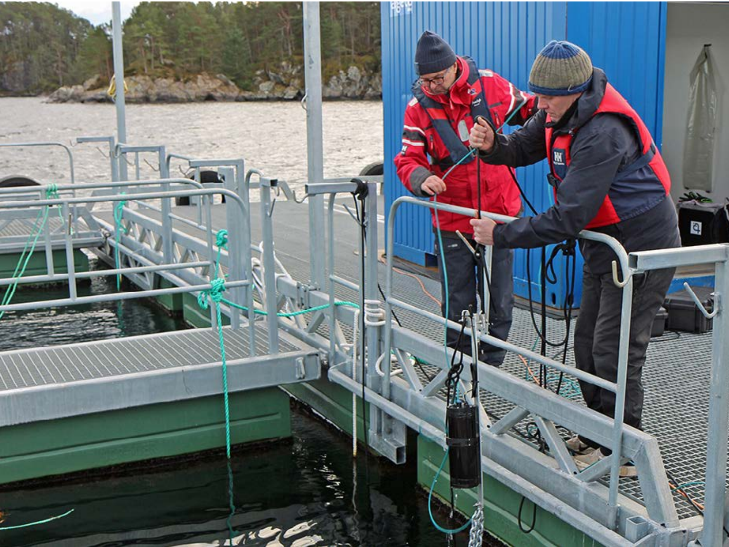
NORCE performed a successful test of their SDM modem in sea for the first time at the marine facility at Austevoll. PHOTO: INGVAR HENNE
