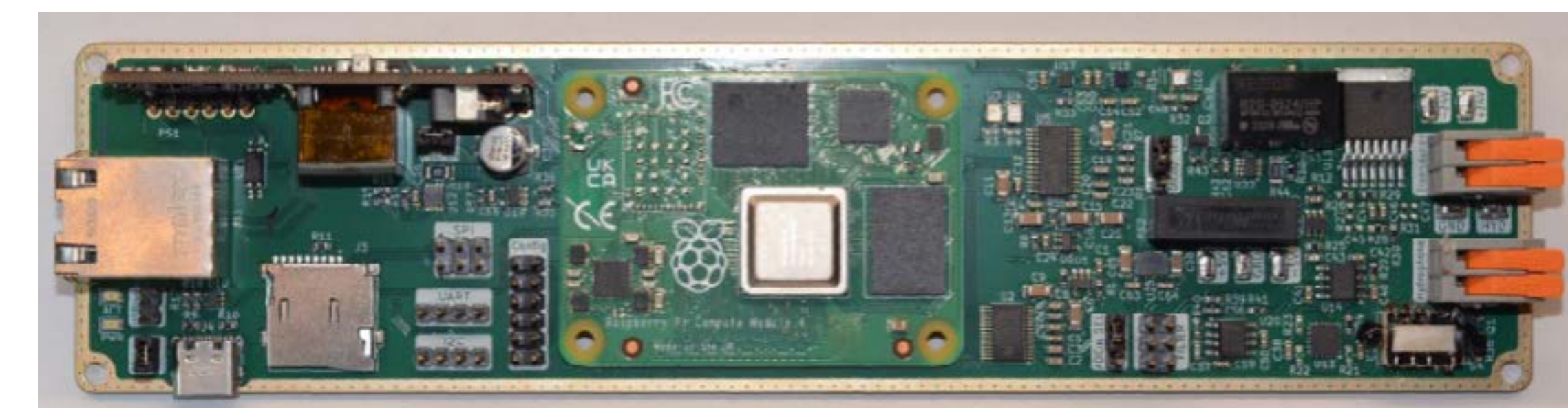
SDM hardware (Steffen Troy, Master's thesis, UiB 2025, design of MARLIN, a test platform for underwater communication) PHOTO: NORCE
