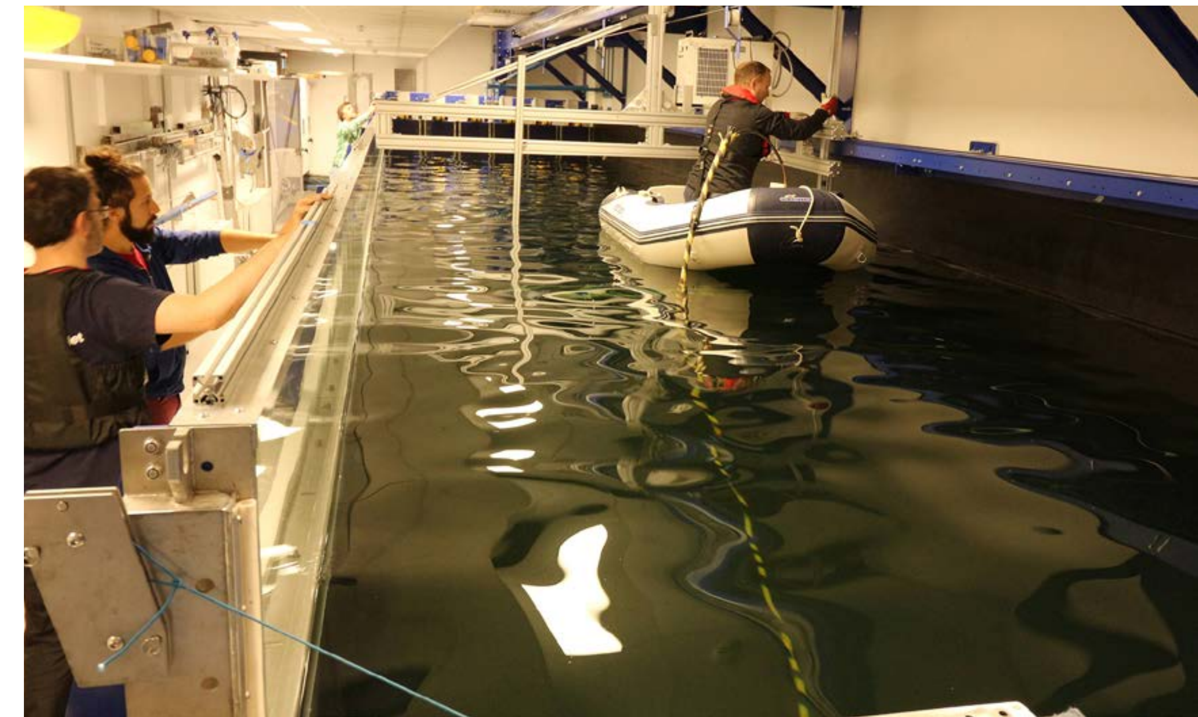
Laboratory tests for DAS at HVL using a subsea telecom fibre cable (cable donated by Tampnet). PHOTO: INGVAR HENNE
